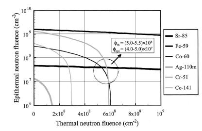
**Fig. 8.** Estimation of thermal and epi-thermal neutron fluences in chemical reagents. The lines of <sup>51</sup>Cr, <sup>59</sup>Fe, <sup>110m</sup>Ag and <sup>141</sup>Ce do not cross each other.
