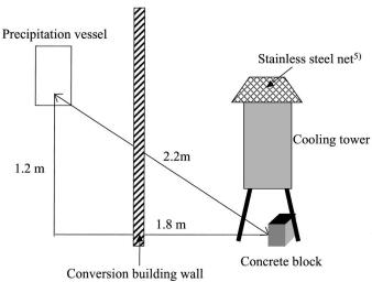
Fig. 3. Schematic view of the sampling point of a concrete block.
