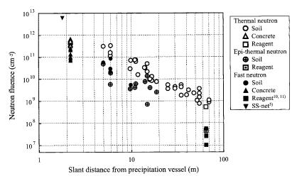
**Fig. 9.** Plots of the thermal, epi-thermal and fast neutron fluences estimated from the soil, concrete-block and chemical-reagent samples as a function of the slant distance from the precipitation vessel.
