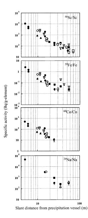
**Fig. 5.** Plots of specific activities of <sup>46</sup>Sc, <sup>59</sup>Fe, <sup>60</sup>Co and <sup>24</sup>Na against the slant distance from precipitation vessel, whose data is separated by 8 directions. , NW direction; , NE direction; , E direction; , S direction and , SW direction.
