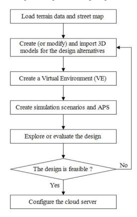
Figure 2. The working process of Cloud Server
