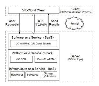
Figure 1. The framework of Cloud-based VR Platform
