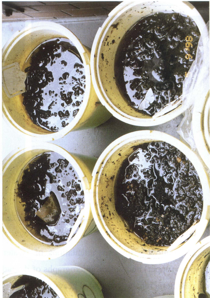
Figure 26 "Water - oil - sediment interaction" experiments inside of building (left) and outside (right) (May 9 th , 1998).
