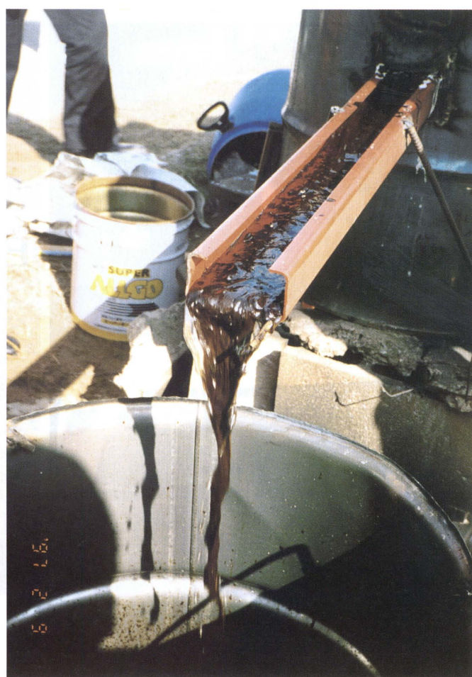
Figure 19 Separation tasks of heavy oil and sands or gravels on the site. Warming up seawater in about 40 °C , adding contaminated sands or gravels, then getting the oil on the surface.
