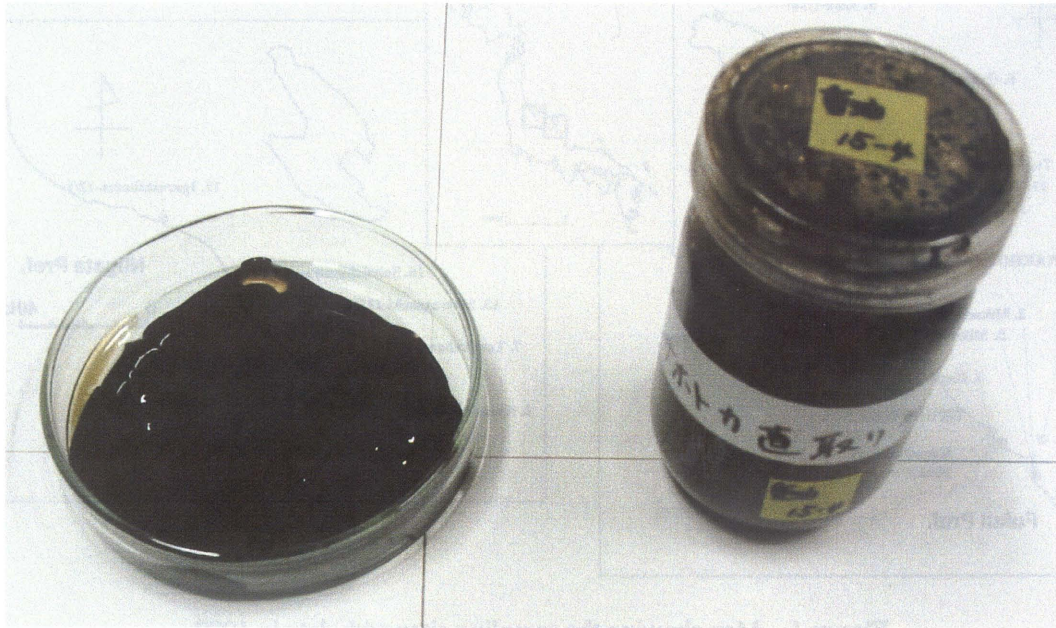
Figure 2a The heavy C oil NAKHODKA-1997/2/6 taken directly from a stem part of the oil tanker sunk near Mikuni.
