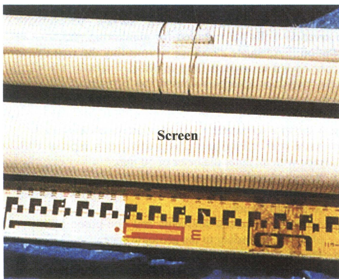
Fig. 9 Casing and Screen
