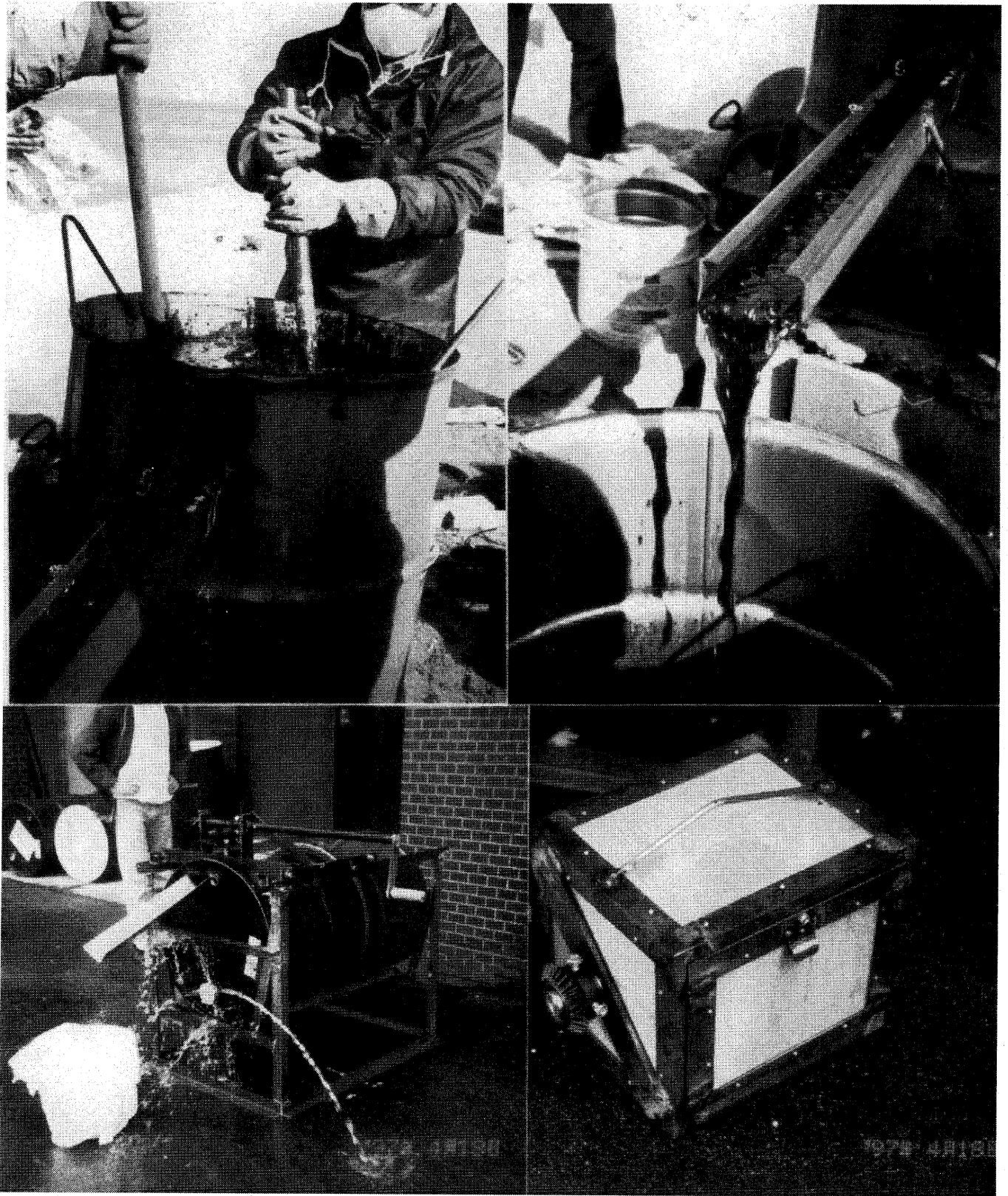
Figure 2 Simple cleaning methods to rinse the polluted beach and gravel was by using the warm seawater. This method effectively removed oil from beach materials. This method and the home made cleaning machines were our idea on February 9 th (upper) and on April 18 th , 1997.
