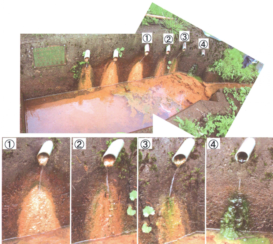
Fig. 2 Field views of biomats in drainpipe outlet at the landslide area in Takayanagi showing light reddish brown biomats (①), reddish brown biomats (②), greenish brown biomats (③), and green biomats (④).
