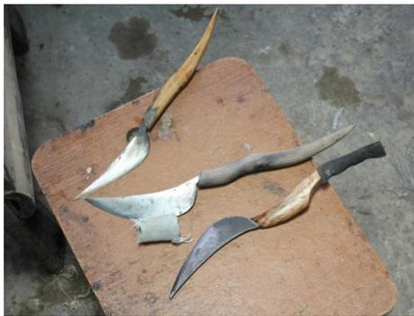
Small knives for cut and slicing bamboo
