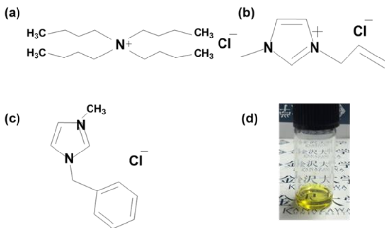
Figure 4.1. Chemical structure of different ILs of (a) [TBAM][CL], (b) [AMIM][CL], and (c) [BMIM][CL]; (d) mixture solution of CH 3 NH 3 PbI 3 and 3 wt % of IL.
