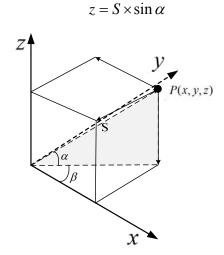
Figure 2-1 3D spatial coordinates of measuring point P(x, y, z)
