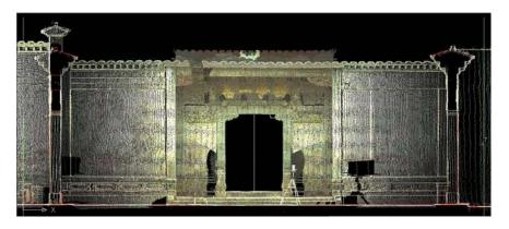
Figure 2-6 The drawing of the entrance vertical face section from the point clouds
