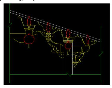
$Figure\ 2\text{-}15\ The\ profile\ drawing\ of\ the\ Dougong\ beams\ above\ the\ Gold\ Pillar$
