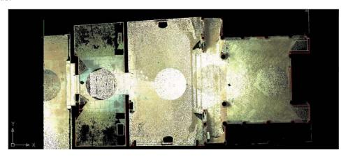
Figure 2-5 The drawing of the entrance plane section from the point clouds
