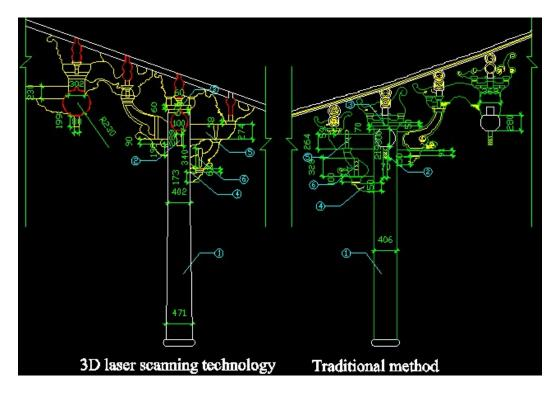
Figure 2-16 Comparison of mapping results of 3D laser scanning technology and traditional method in detailed components
