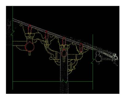
Figure 2-14 The drawing of the Dougong beams above the Gold Pillar using the point clouds
