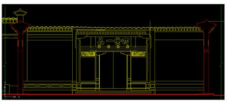
Figure 2-9 The vertical face drawing of the entrance
