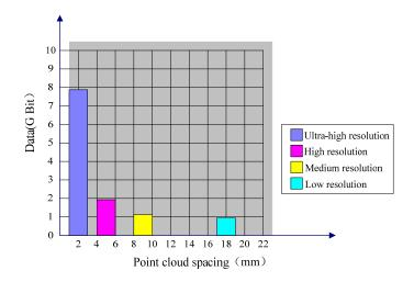
Figure 2-18 The spacing and data of one site's data point cloud at different scanning resolutions
