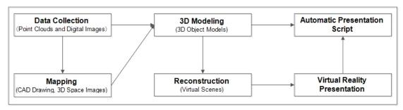
Figure 2-2 The flow chart of virtual reality presentation based on 3D laser scanning technology
