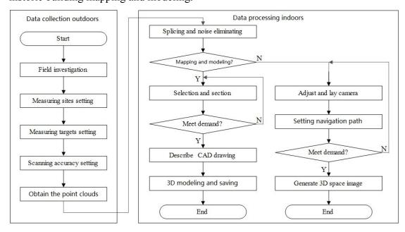
Figure 2-3 The flow chart of 3D laser scanning technology for historic building mapping and modeling
