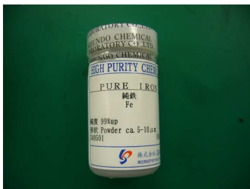
Fig. 2-21 \alpha Fe powder.
