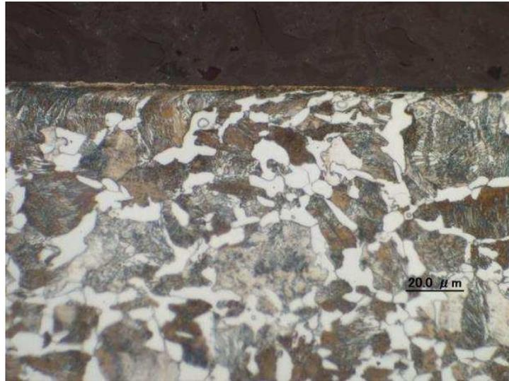
Fig. 2-23 Microstructure of the S45C test piece.
