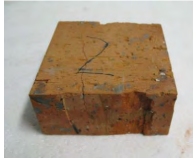
Photo 4.1. Bricks specimen for compression test.
