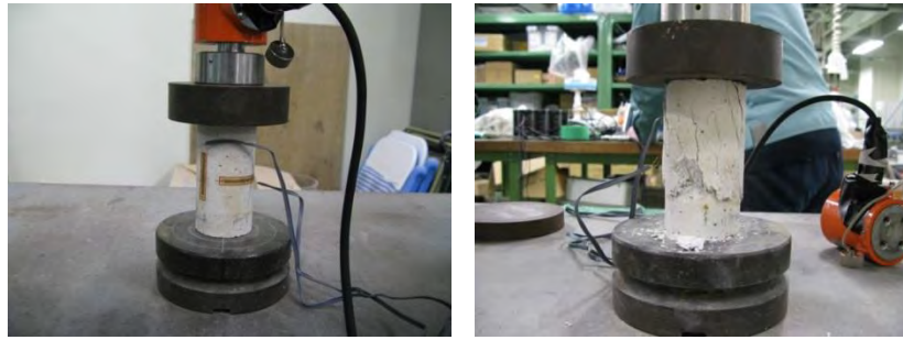
Photo 4.2. Mortar compression test and failure mode.
