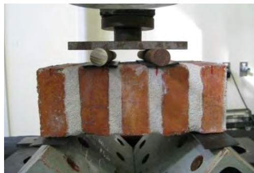
Photo 4.5 Specimen test setup for flexural bond test.
