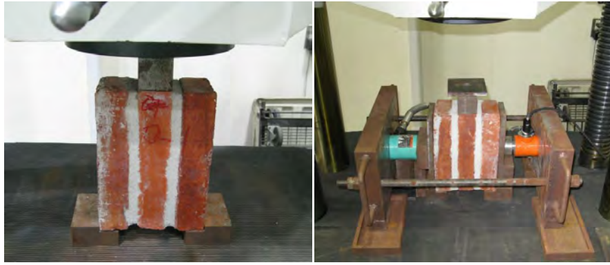
Photo 4.6. Triplet test setup for shear test on masonry prisms.
