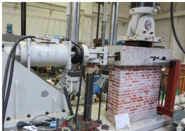
Photo 4.10. Loading system in cyclic test.
