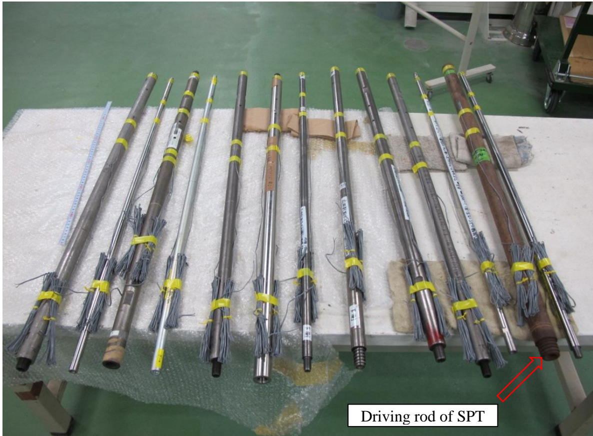
Figure 6.2. Various types of driving rods of DCPTs and SPT instrumented with strain gauges
