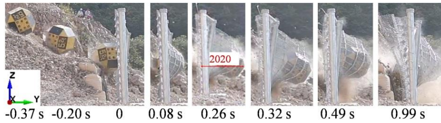
Figure 2.9 Behavior of the rock fence (Test No. 2)
