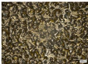
(a) Optical microscope image of consolidated surface before wire cut
