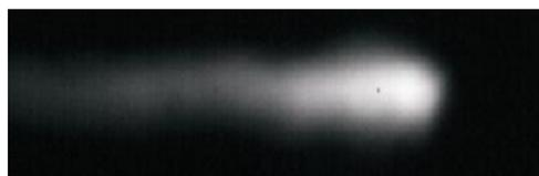
Fig. 5.3 Typical image of SLM melt pool from high-speed camera [5]
