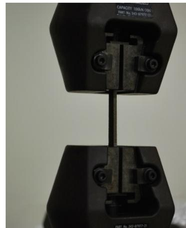
(b) Specimen during tensile test
