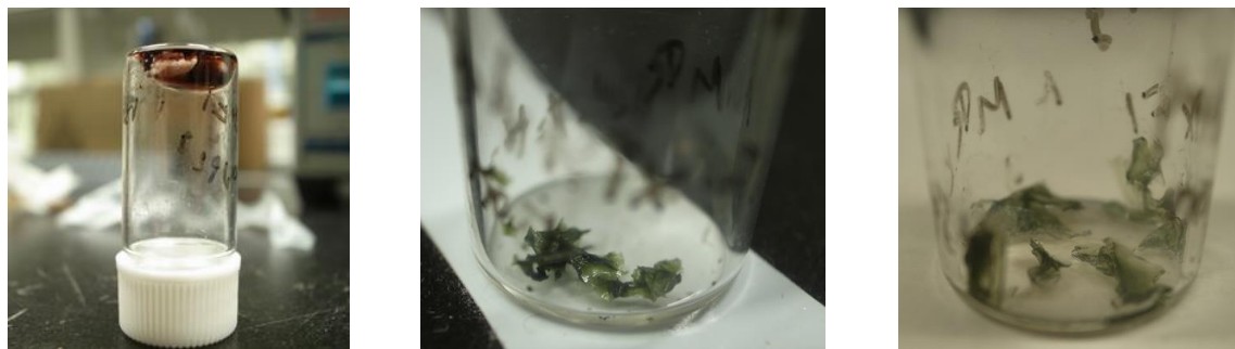
Figure 4-14. Image of topological gel. (a) Gelation of polyRTX-2, (b) dry topological gel and (c) wet topological gel with chloroform.
