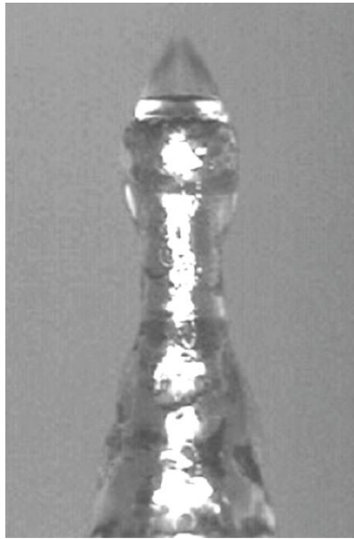
Fig.5-2 Diagram of the top of an electrostatic atomizer.
