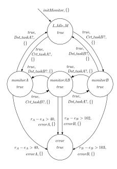
Figure 4: Monitor automaton checking schedulability
