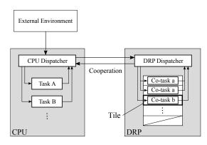
Figure 2: Overview of the CPU-DRP embedded system
