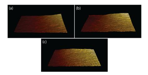
Figure 4: Snapshots of 44 successive contact-mode AFM images of calcite crystal dissolution process in water. (a) 0 s. (b) 40 s. (c) 80 s. Scan size:  $20 \times 10 \text{ nm}^2$ . Scan rate: 50 Hz. Imaging speed: 2 s/frame. Pixel size:  $200 \times 100 \text{ pix2}$ . Tip velocity: 4 µm/s.  $f_{cr} = 5.8 \text{ kHz}$ .
