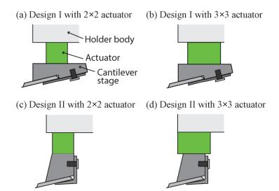
Figure 2: Schematic models of the Z tip scanners with different designs of a cantilever screw holding mechanism
