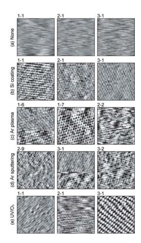
Figure 5: FM-AFM images of a cleaved mica surface obtained in PBS solution. (a) None. (b) Si coating. (c) Ar plasma. (d) Ar sputtering. (e) UV/O3. The numbers n-m indicated in each image shows that the image corresponds to the m-th image obtained in the n-th experiment. Scan size:  $8 \times 8 \text{ nm}^2$ . Tip velocity: 223 nm/s. A = 0.25 nm.  $\Delta f = 800 \text{ Hz}$ .
