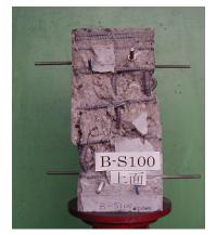
At the stage of Photo 6.4: View of experiment and specimens after loading cover concrete peel of commencement:
