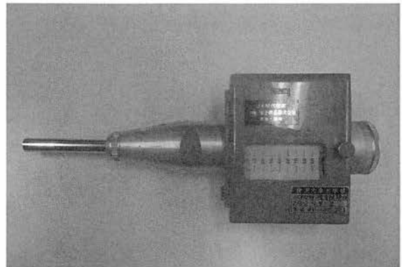
Fig.1 Schmidt hammer used for measuring surface hardness of rock walls at the churches
