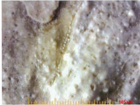
Fig. 15 Microscopic image of the middle of fig. 14. This is a part of nose boundary (small white dots in line) of No.3 on fig. 3(a)
