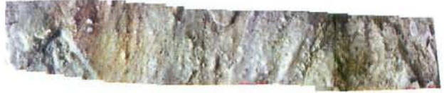
Fig. 14 Synthesis microscopic image of the region No.3 on fig. 3(a) consisted of images by sequential scan imaging.
