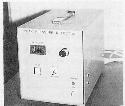
Fig. 2 The box of strain amplifier and force calculator
