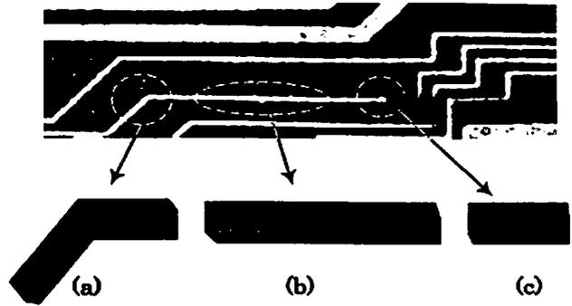
Fig. 1: PCB pattern could be separated into many basic parts such as: (a) open elbow, (b) straight, and (c) half part.
