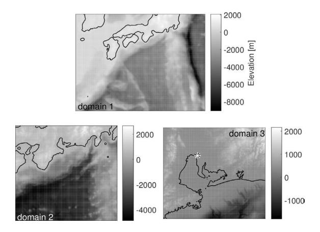
Fig. 3 Computational domains 1–3 used in storm surge modeling (\* is Nagoya Port location).
