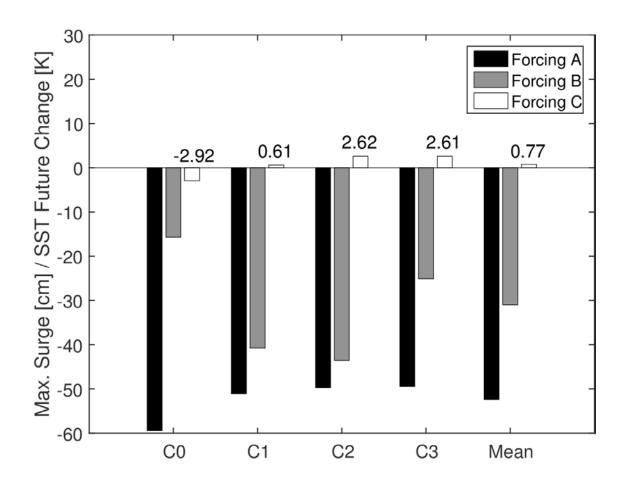
Fig. 14 The ratio of changes in storm surge due to PGW experiments to averaged SST in the Western North Pacific.
