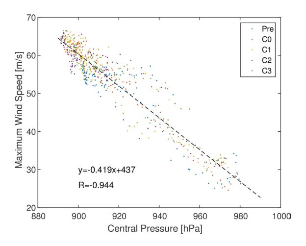
Fig. 5 Relationship between central pressure and maximum wind speed of typhoon.
