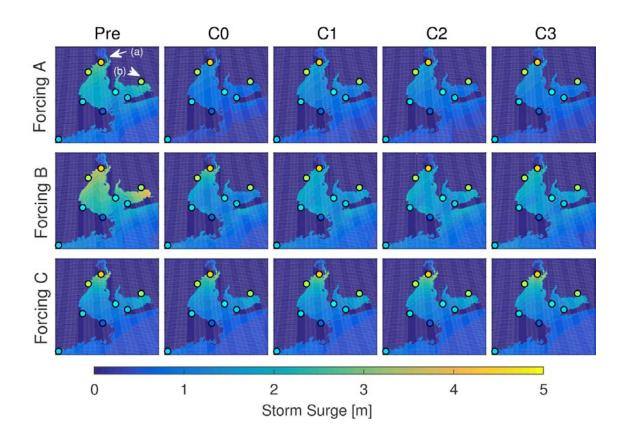
Fig. 10 Distributions of maximum storm surge height (top panels: forcing condition A; middle panels: forcing condition B; bottom panels: forcing condition C; columns (left to right): Pre, C0, C1, C2, and C3); color scale: the surge height in meters; circle: observed surge height at the locations; (a) and (b): locations of Nagoya Port and of innermost of Mikawa Bay corresponding to Table 4.
