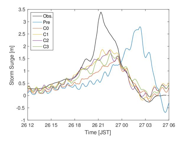
Fig. 11 Time series of storm surge height at Nagoya Port for the Pre and PGW experiments with forcing condition A as well as the observed surge height.
