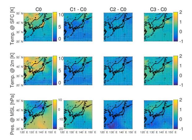
Fig. 2 In the SST ensemble experiments, future changes in surface temperature [K] (top row), in near-surface air temperature [K] (middle row), and the pressure at mean sea level [hPa] (bottom row) (left-most column: baseline condition C0; other columns: difference from C0).
