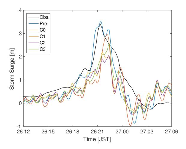
Fig. 12 Time series of storm surge height at Nagoya Port for the Pre and PGW experiments with forcing condition B as well as the observed surge height.
