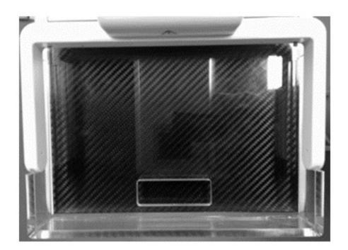
Customized compression plate. We pierced the compression plate such that the center was at a position 3.5 cm from the chest wall, an area through which an ultrasound probe was to be placed.
