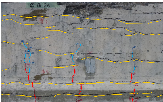
Fig. 16 Crack pattern at the span center after loading test.
