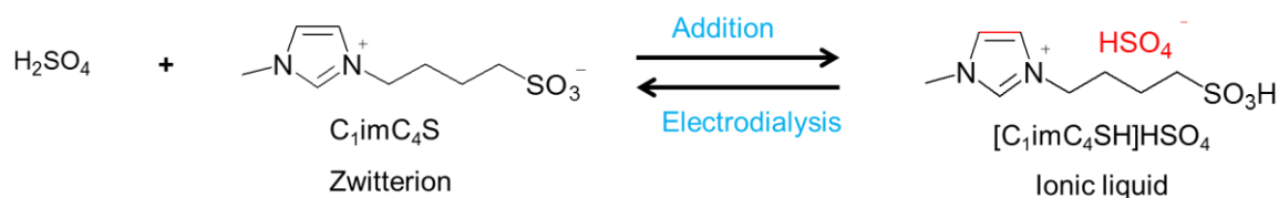
Figure 3- 6 Reaction of in situ synthesize [(C 1 imC 4 SH)]HSO 4 from H 2 SO 4 and C 1 imC 4 S and reversible separation of [C 1 imC 4 SH]HSO 4 into the components by electro dialysis
