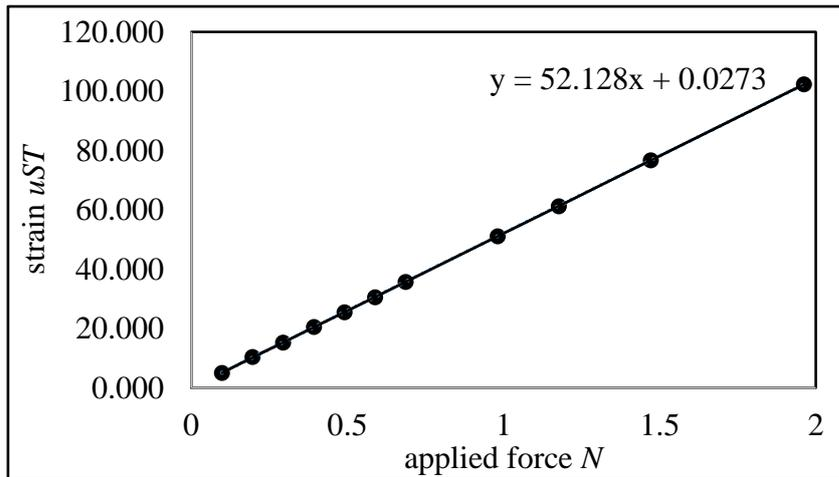
Figure 3.5. Load cell calibration result
