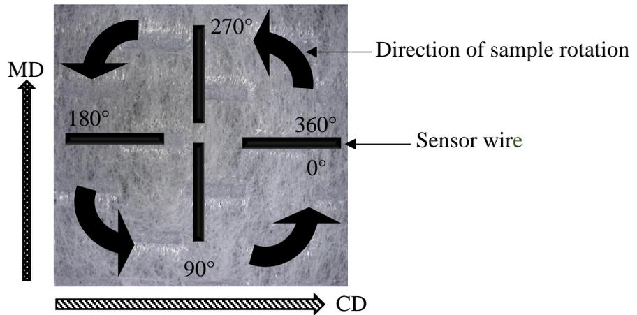
**Figure 4.7. The relative positions of sensor wire in different directions of test**
