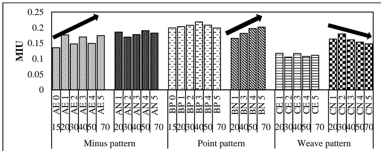
**Figure 5.7. Effect of fabric density on MIU values**
