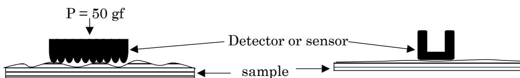
**Figure 5.1. Detector for surface friction test**
