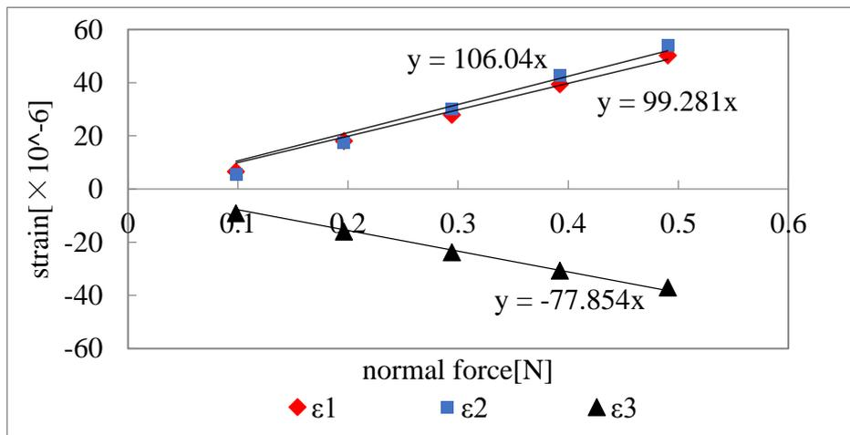
Figure 3.6. (a) Tactile sensor calibration (Normal force)
