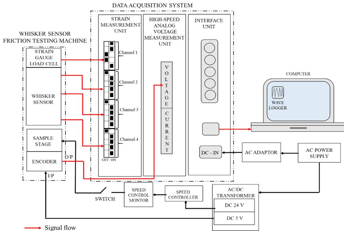
**Figure 3.2. Block diagram of whisker type tactile sensor friction testing machine**
