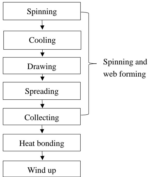
**Figure 4.1. Flow diagram of spunbond process**
