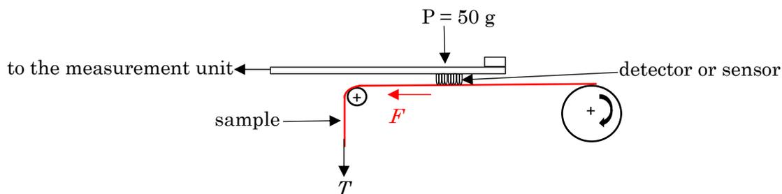
**Figure 2.3. Kawabata surface friction tester**
