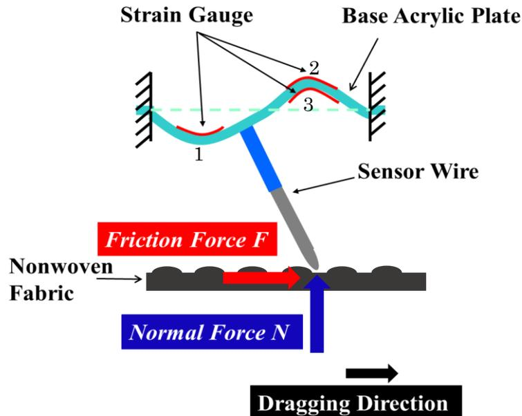
**Figure 3.4. The working principle of sensor**
