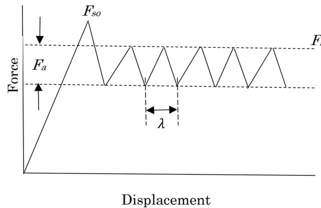
**Figure 2.5. Hypothetical friction trace for a textile material**
