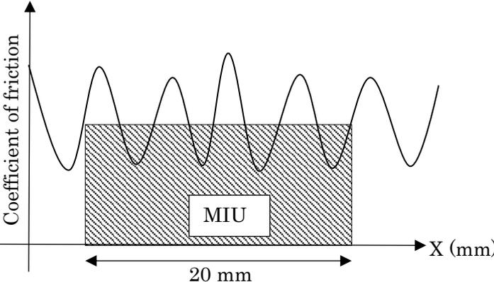
Figure 5.2 (a) Surface friction (MIU)
