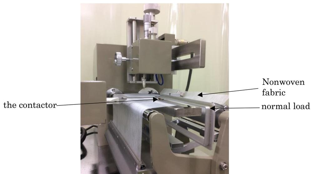
**Figure 5.3 Surface friction and roughness tester (KES-FB 4)**
