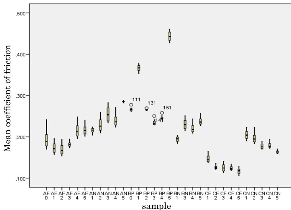
**Figure 4.11. Box-plot for spunbond nonwovens**
