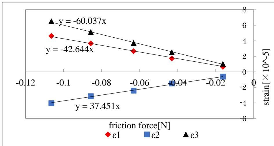
Figure 3.6. (b) Tactile sensor calibration (Friction force)
