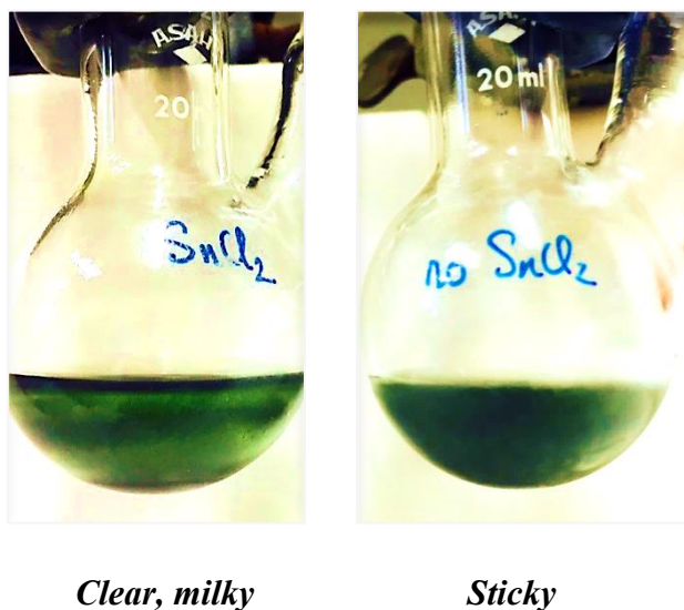
Picture 3.1. The reaction mixture with and without \text{SnCl}_2 . Reaction Conditions: \text{PdCl}_2 , \text{Cu}(\text{MeCN})_4\text{BF}_4 , DABCO, \text{CO}/\text{O}_2 (ca, 1/1, 1 atm), \text{MeOH}/\text{THF} (v/v = 1/1), 50^\circ\text{C} , 3 h.
