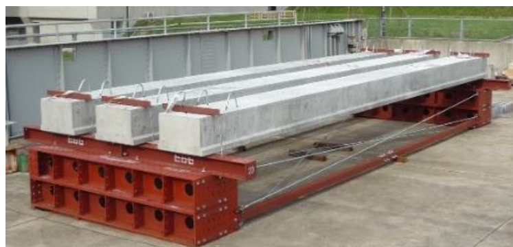
Figure 1 Exposure condition of the PC girders at Kakuma campus
