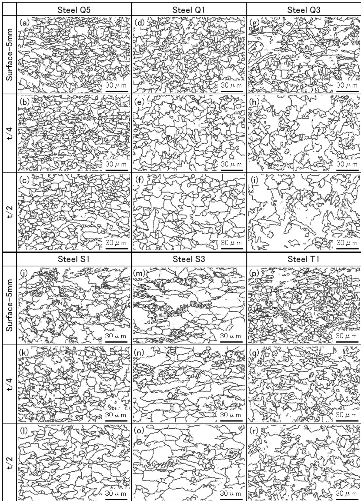
Fig. 4-6. EBSD grain boundary maps of Steels Q1, Q3, Q5, S1, S3 and T1 (Misorientation \geq 15^\circ ).
