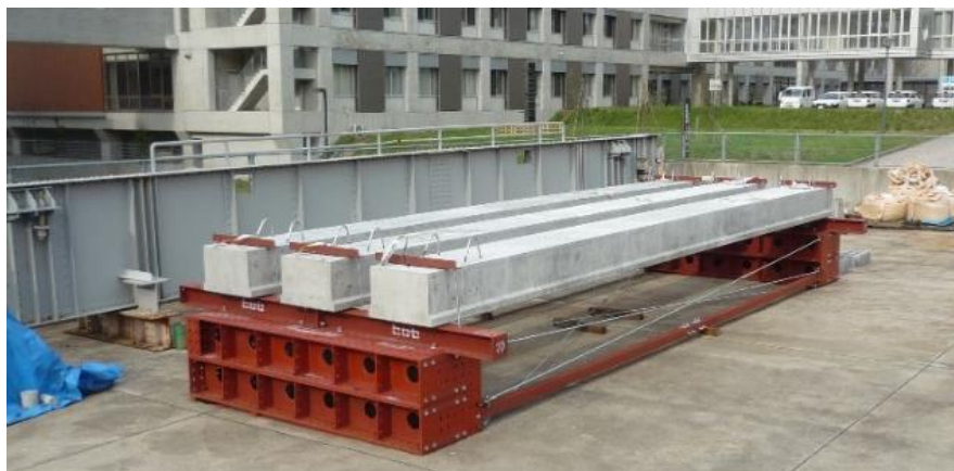
Figure 2.3 Exposure condition of the PC girders at Kakuma campus
