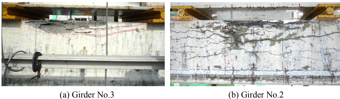
Figure 2.13 Compressive failure mode at the span center of girders at the final loads.
