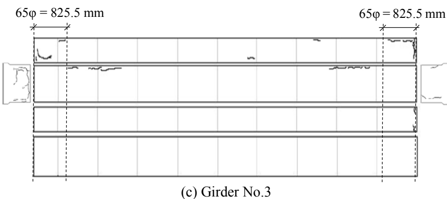
Figure 2.4 Crack patterns of the three girders (From top to down: north side surface, top surface and both surfaces near both ends, south side surface and bottom surface) and the adhesion transmission length of tendons (approximately 825.5 mm) (unit: mm).
