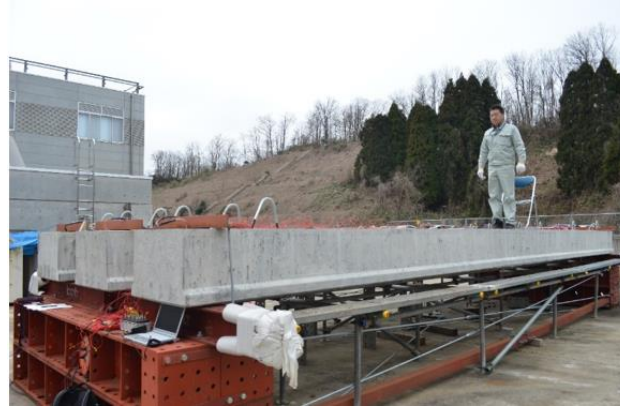
Figure 4.2 Impact test and sensor layout on the PC girder.
