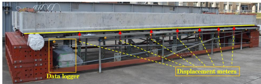
Figure 5.4 Measured point layout under the PC girder (Unit: mm)
