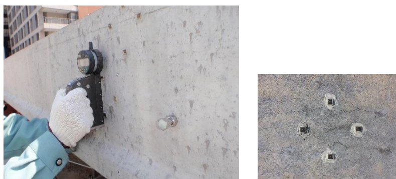
(a) Contact micron strain gauge (b) Gauge chip setup
