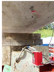
(a) Wire displacement meters
