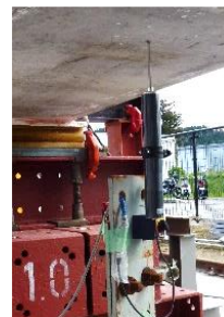
(b) High-sensitive displacement meters
