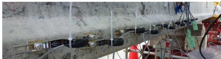
(c) Pi-shaped displacement gauge
