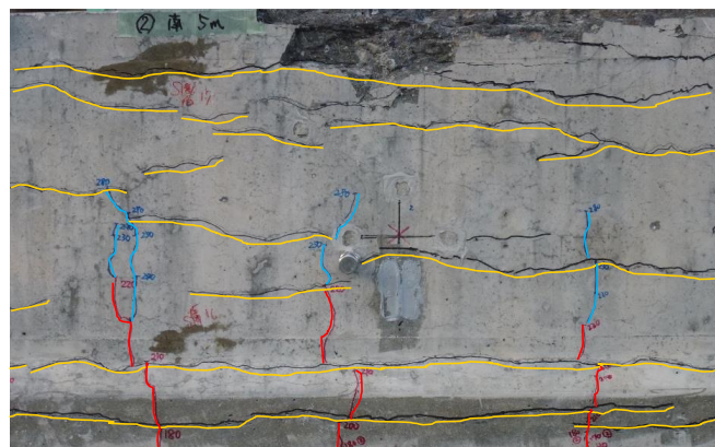
Figure 2.16 Crack pattern at the span center after loading test.
