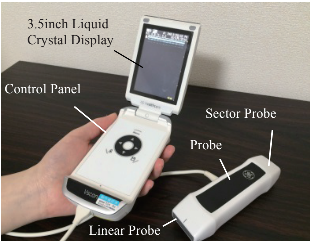
Figure 1. The portable ultrasound diagnostic imaging device used in this study The body of this pocket ultrasonography is foldable and palm-sized. Linear and sector probes are mounted on each end of the probe.
