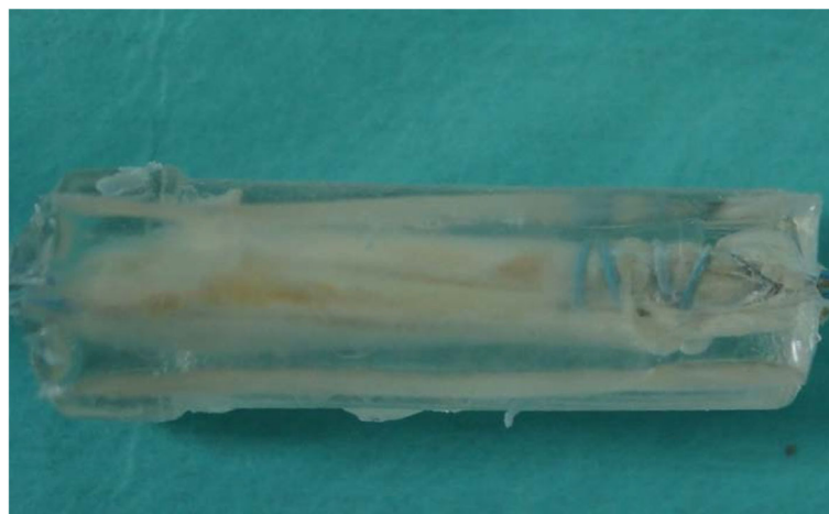
Fig. 4 How to fix the graft. a The graft was dipped in a mold filled with resin and irradiated with ultraviolet light for three minutes. b The fixed graft with Ultraviolet-curing acrylic resin
