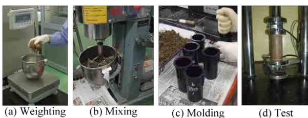
Fig.1 Overview of soil test
