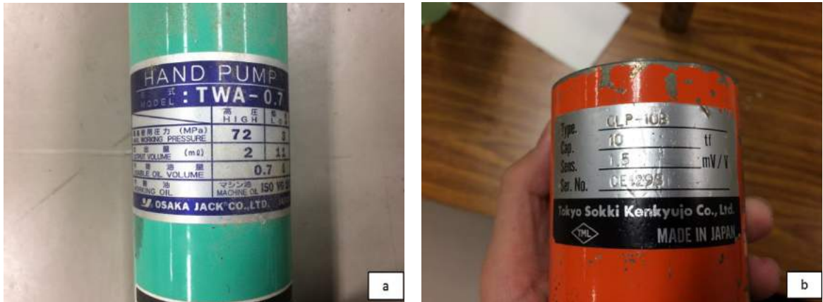
Figure 3.8 Instruments used in the pull-out test; (a) Hydraulic jack, (b) Load cell
