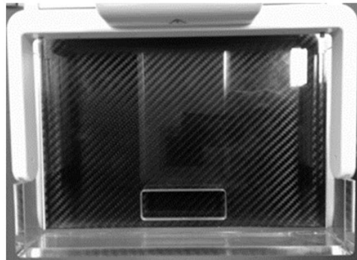
Fig. 1 Customized compression plate. We pierced the compression plate such that the center was at a position 3.5 cm from the chest wall, an area through which an ultrasound probe was to be placed.
