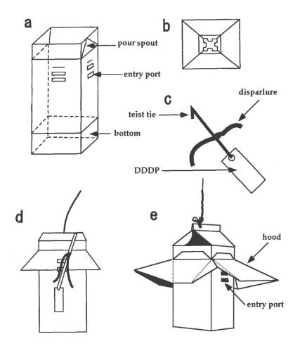
**Fig. 1. A gyspy moth milk carton trap used in this research.** a: Trap body. b: Trap hood. c: Internal chemical agents (a (+)-disparlure wick and with a DDDP strip). d, e: Assembled Trap
