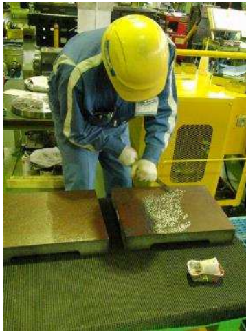
Photograph of scraping the surface of the platen
