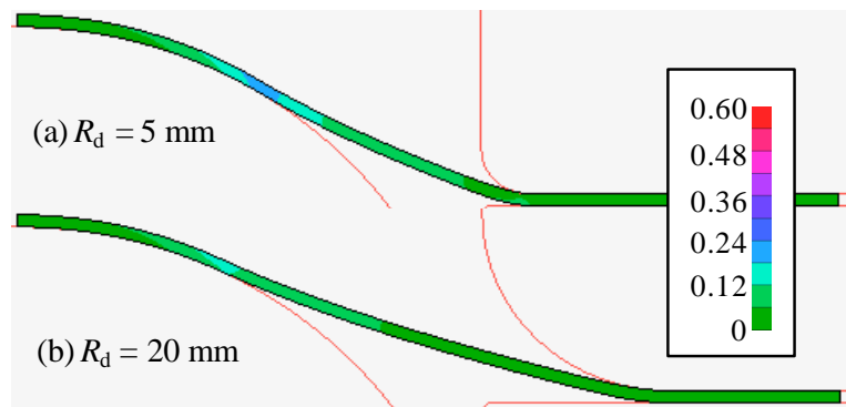
Fig. 3-18 Effect of R_d on distributions of equivalent strain calculated by finite element simulation for T_s = 800 °C, V = 8.1 mm/s and H = 20 mm
