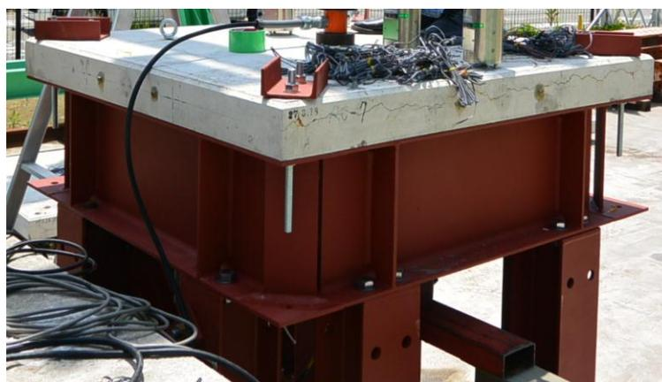
**Figure 3.4** The steel frame for FWD experiment
