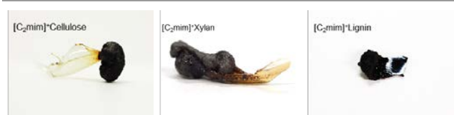
Fig. 3 Char formation of the thin films of [C 2 mim] + cellulose (left), [C 2 mim] + xylan (centre), and [C 2 mim] + lignin (right) after burning and extinguishing the fire.
