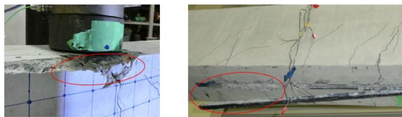
(a) Concrete fragmentation (b) Peeling of FRP bar
