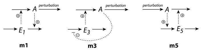
**Fig 1.** The negative feedback loops m1, m3, and m5 used in this study. Solid arrows indicate reactions/mass flow, while dashed lines indicate activating or inhibiting signaling events. *A* is the controlled variable, which is kept at a certain set-point by opposing (step-wise) perturbations in *A*. The *E*<sub>*i*</sub>'s are controller species.
