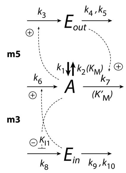
**Fig 3. Combination of controller motifs m3 and m5 with** *A* **as the controlled variable.** Rate parameters  $k_1$  and  $k_2$  are perturbations.  $K_M$  and  $K'_M$  (in parentheses) are used when zero-order degradations with respect to *A* are studied and controllers become oscillatory (see next section).  $K_{I1}$  is an inhibition constant.
