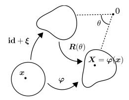
Figure 1: Sketch of the reference domain  $\overline{\Omega}$  and the deformed configuration  $\varphi(\overline{\Omega})$ .
