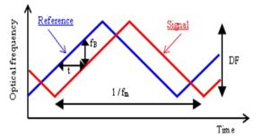
**Figure 2**. The waveform of the optical Frequency.
