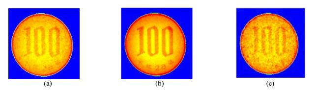
**Figure 8.** The image profile of 100 JPY coin using asymmetric method with the frequency modulation (a) 2.1 kHz; FFT 8192 in 21.769 s (b) 1.8 kHz; FFT 4096 in 23.134 s (c) 2.5 kHz; FFT 4096 in 17.551 s.
