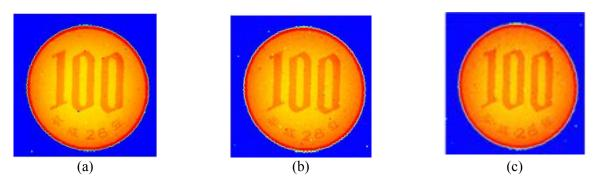
**Figure 6**. The image profile of 100 JPY coin using symmetric method with the frequency modulation (a) 0.5 kHz FFT 8192 (b) 1.2 kHz FFT 4096 (c) 1.4 kHz FFT 4096.
