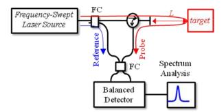
**Figure 1**. Basic configuration of FMCW optical sensing system.
