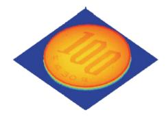
Figure 4.12 Three-dimensional profiling result of a Japanese 100YEN coin without optimizing timing for  $f_m = 1$  kHz.
