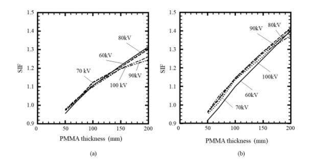
Fig. 2. SIF variations as a function of PMMA thickness using (a) G6 and (b) G10.
