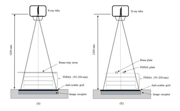
Fig. 1. Schematics of acquiring geometries for measurements of (a) scatter fraction (SF) and (b) signal-difference-to-noise ratio (SDNR).
