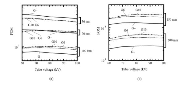
Fig. 4. Results of tube voltage dependencies in figure of merit (FOM) calculated as SDNR<sup>2</sup>/ESAK (SDNR: signal-difference-to-noise ratio, ESAK: entrance surface air kerma), for the bone contrast with (a) 50-, 70-, 100-mm thicknesses, and (b) 150- and 200-mm thicknesses.
