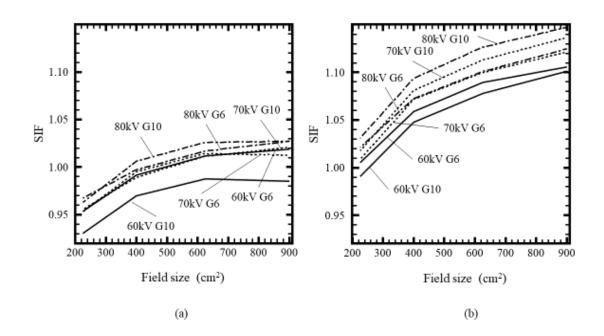
Fig. 3. SIF variations as a function of field size for (a) 70-mm and (b) 100-mm thicknesses.
