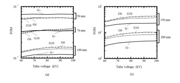
Fig. 5. Results of tube voltage dependencies in the FOM for the PMMA contrast with (a) 50-, 70-, 100-mm thicknesses, and (b) 150- and 200-mm thicknesses.
