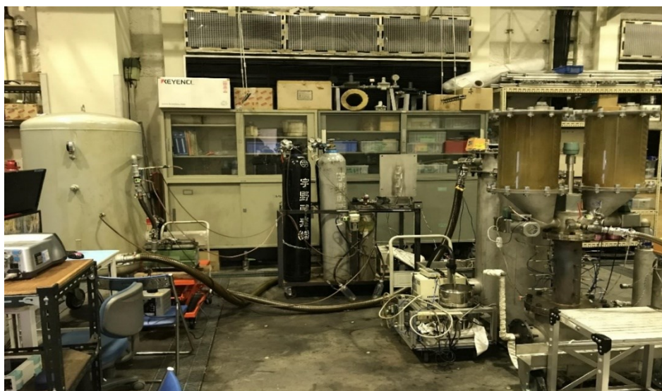
Figure 27. Real of Downdraft Gasifier System Equipment
