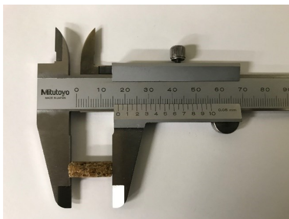
Figure 22. Wood Pellet Specification: Length of Wood Pellet Feedstock
