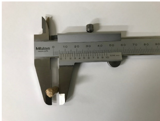
Figure 21. Wood Pellet Specification: Diameter of Wood Pellet Feedstock
